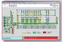
The visualisation system ViSIT, developed by SITLog, has the whole material flow plant under control. No matter if HBW, MLS, individual conveyor module or picking area - ViSIT records - freely selectable by time unit or plant area - , for instance where and which event led to a reduction of the performance.
