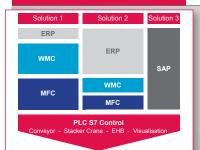
SITLog controls, coordinates and manages different warehouse logistics systems in distribution, production and manufacturing with the modular systems SITLog WMC and SITLog MFC.
